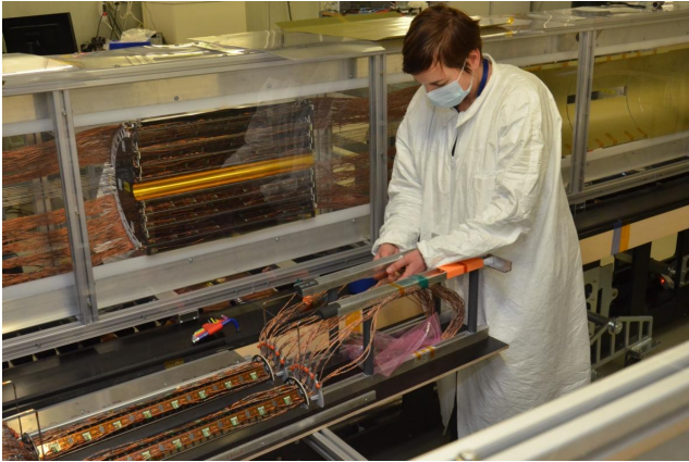
Half-disk electronics of the TEPX detector with 26 modules undergoing tests in a climate chamber. The CMS TEPX detector will consist of 1408 detector modules.
