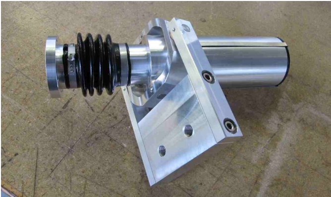
FIG. 15.4 – Masterpiece from Brandon: mirror actuator for CTA.
