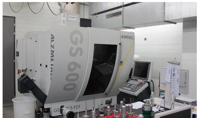
FIG. 15.3 – New high-performance, milling - turning and machining centre. The top figure shows the transport through the corridor.
