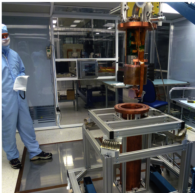
The copper box hosting the CCDs, top lead shield and in-vacuum electronics being inserted in the copper vacuum vessel.
