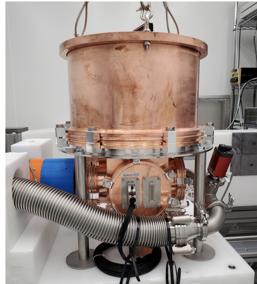
The new prototype DAMIC experiment, being installed in the Modane underground laboratory in France in November 2021. Shown are the copper box housing the CCD detectors, as well as lead and polyethylene shielding.
