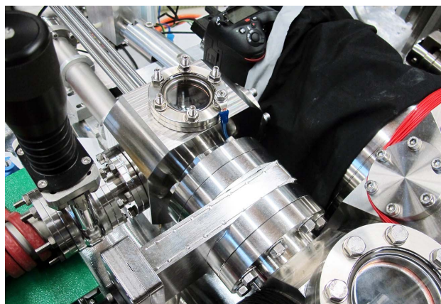
- Load-lock system enabling the rapid transfer of samples into the UHV chamber. An additional port permits the electro-spray deposition of biomolecules onto ultra-clean freestanding graphene.
