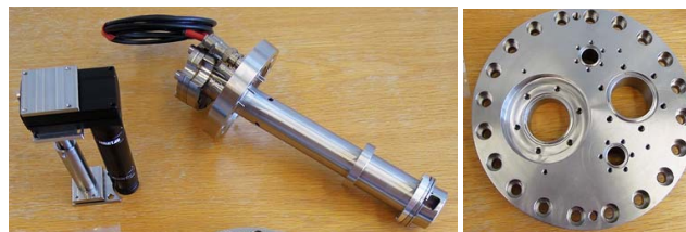
- Parts of an electron diffraction experiment. Electrons back-reflected by a sample produce light on a phosphorous screen after amplification by a micro channel plate. These parts are mounted inside a tube, seen in the middle. The screen is imaged through a vacuum viewport onto an external CCD, seen on the left. The picture on the right shows the detector flange.
