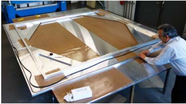
- Manufacturing of large parts for the FlashCam camera housing on a special table installed in the lock-smithery of the workshop
